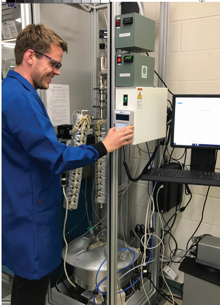
Reactive distillation apparatus used for the RAPID project at Sironix HQ in Seattle
